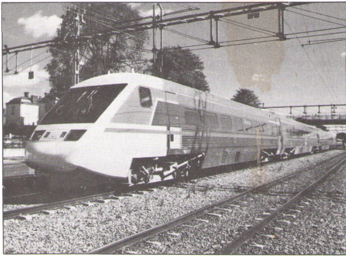
Late this year, Amtrak will test a Swedish X-2000 tilt train (modified to meet FRA safety requirements). When the consist runs outside electrified territory, an Amtrak turbine will replace the sleek X-2000 power unit. At a Nov. 21 news conference, Amtrak Pres. W. Graham Claytor Jr. said electrification and tilt technology together could produce 3-hour Boston-New York running times; tilt could even reduce New York-Washington times "to some extent."
